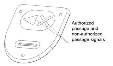
Fig. 2 General view LED panel display
