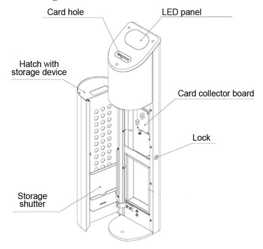
Fig 5. General view of card collector
