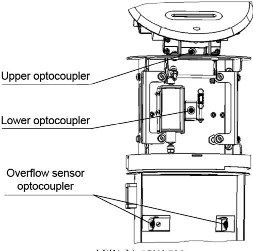
LED(r/b) L7113 F3C Optotransistor (y/b) L7113 Fig 7. Location of optocouplers of card reader
