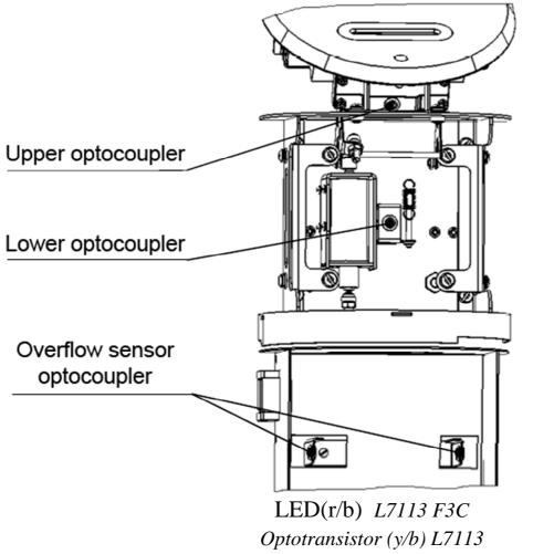
Fig 6. Location of optocouplers of card collector
