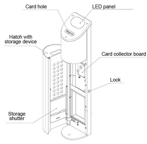
Fig 4. General view of the card collector
