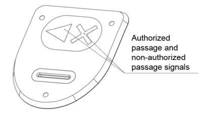
Fig. 2 General view of LED panel
